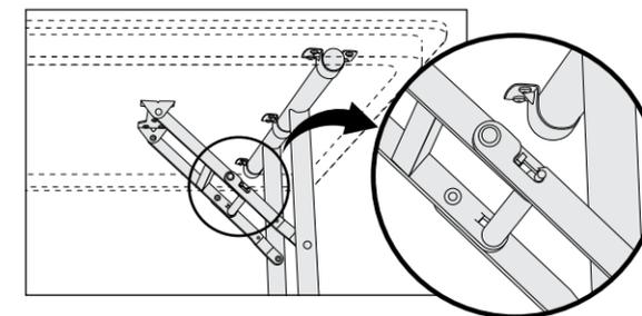
Virco's patented locking mechanism adds strength, security and convenience to our wishbone and C-leg designs. When setting up tables, simply unfold each leg with an outward motion to extend the hinges and engage the gravity-lockpin. To return legs to a folded position, set the table on its side and push the gravity-lockpin toward the table top, disengaging the pin from its locked position and allowing you to easily complete the folding process.
