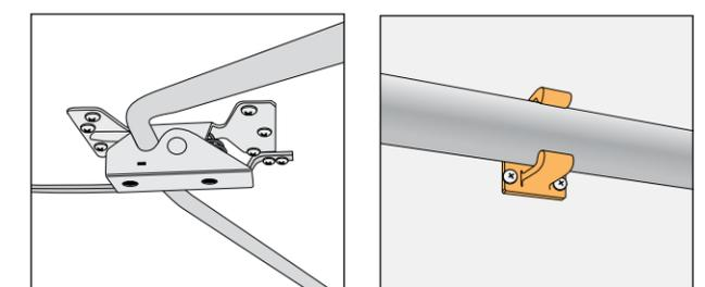
Round Core-a-Gatortables have a convenient spring clip mechanism that securely locks unfolded legs in position (left). Folded legs are held in place by injection-molded retention clamps for safe transport and storage (right).
